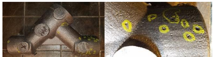
Inclusions Marked for Repair
