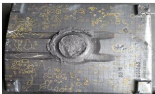
Inclusions Marked for Repair on Casting Cope Surface
